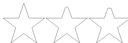
Transform>Fillet Round Corner (Setting of 0.08; middle image : no miter, right image : miter checked; Individually click on which interior or exterior corners you wish to fillet)
