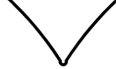
Trailing Blade is too high: Divots will appear around corners
