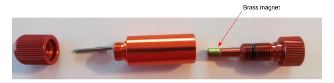
(3) The brass part is the magnet. Pull it away from the top of the blade holder and flip it upwards so that you can see the hole where the bottom part of the blade is inserted:
