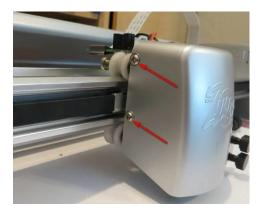
(4) The sensor mount is right on the front, with two screws to hold it. First, have a look at how yours is currently mounted versus my own. Note the green arrows in the following photo show that mine was mounted close to the highest it could go. This position has always worked very well on my Zing Orbit. However, some owners need the opposite (all the way down) or somewhere in the middle:
