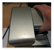
(3) There are two screws on either side of the carriage cover. Remove all four and then set the cover aside.
