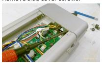
5. Open top cover, remove side cover screws.
