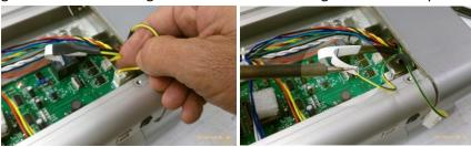
Remove the flat cable: you must unlock the connector before pulling the cable!
