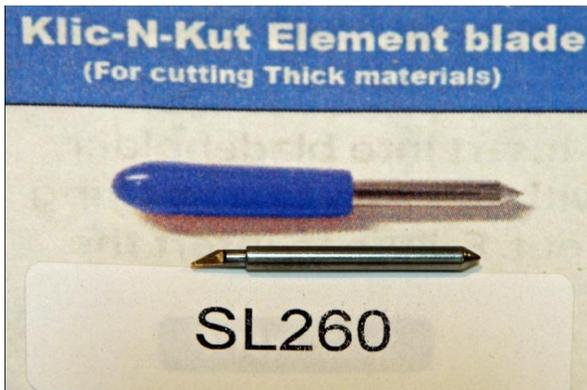
I used the Sliver 2 blade for cutting the clay because it has the longest usable blade length. The maximum thickness of the clay that you can cut cleanly with the KNK is determined by the usable blade length. Because of the thickness of the clay, the blade will most likely be extended to its maximum length.
