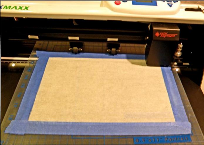
To prepare the mat for cutting the clay, I laid a piece of the parchment paper onto the sticky surface. Since the parchment is coated with silicon, it won't stick securely to the mat and it is necessary to tape the paper down with the blue painter's tape.
