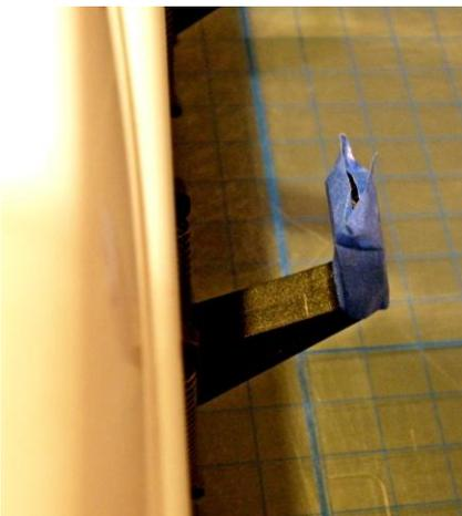
As a reminder to myself to not engage the center pinch wheel, I wrapped the lever with blue painter's tape.
