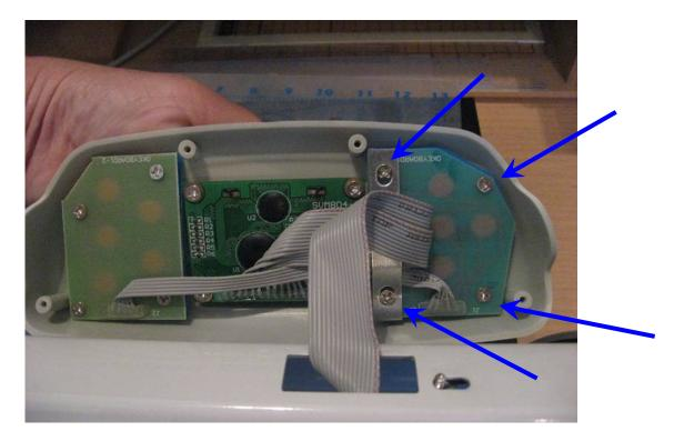
• Using an eraser, rub/clean the five gold circles on the green panel which come into contact with the buttons.
