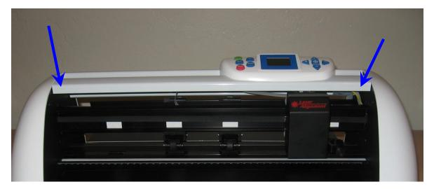
• Remove all four screws under the top (note that mine is the white 15" Maxx whereas you may have the black 24" Maxx or even the handheld control panel on the Eagle.
