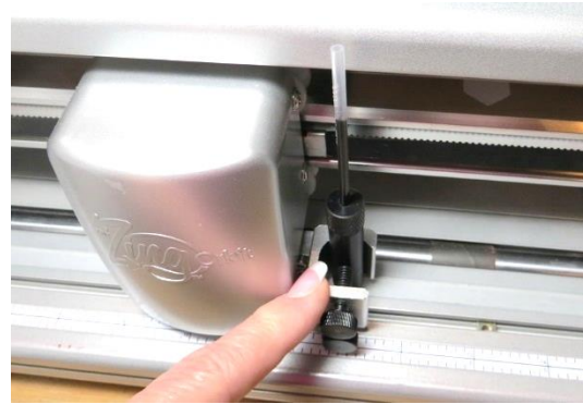
While holding the seat down, insert the test pen and with your other hand tighten the front screws.
