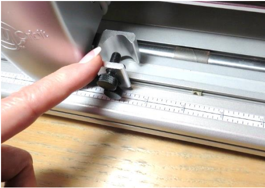
Push the blade holder seat all the way down.
