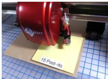
Use 15 with blue blade and for slightly thicker materials
