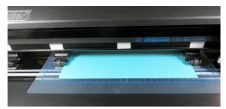
Pinch wheels are approx. the same distance from the outside edges of the cutting mat
