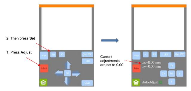
• One at a time adjust  $\Delta x$  and  $\Delta y$  by pressing the buttons in the direction you need the cut line to move.
