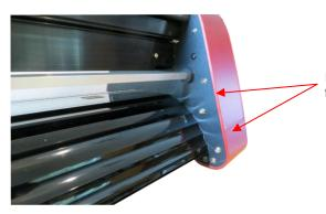
Remove these two screws from right-side end cap
