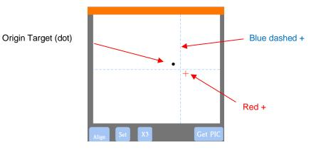
(6) Press the center of the origin target in the photo so that the red + will be moved approximately over it:
