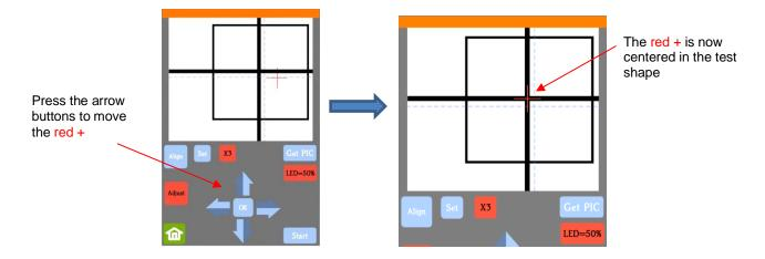
(10) Press **OK** and a new photo will be taken. The blue dashed + should now be more closely aligned with the center of the test shape:
