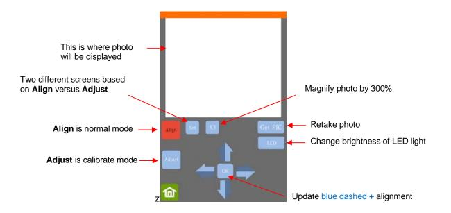
(6) Press **Adjust** to switch to calibrate mode. Press and hold the **OK** button for several seconds until it and the arrows around it turn red (if the buttons do not turn red, please refer to *Appendix D1*):
