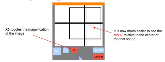
(10) Use the arrows keys to move the center of the red + to the center of the test shape:
