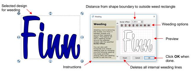
Border Offset: Increase or decrease to set the spacing between the shapes and the outside weeding rectangle. The red line represents that outer cut. For example:
