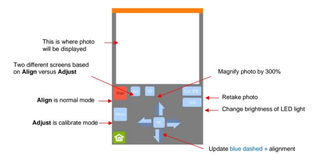
(5) Press Adjust to switch to calibrate mode and a new Start button will appear in the lower right corner of the Camera Screen:
