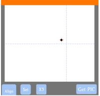
(7) Press **OK**. In the new photo, the blue dashed + should be close to the origin target. Press **X3** to zoom in:
