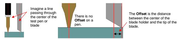
• If you set the **Blade Offset** to 0 when cutting with a blade, corners will be rounded. On the other hand, if it is set too high, bubbles will be cut on sharp corners:
