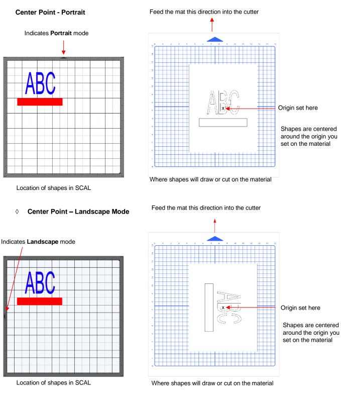
• Note that the alignment is based on the <u>center</u> of the bounding box around the shapes:
