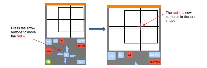
(11) Press **OK** and a new photo will be taken. The blue dashed + should now be more closely aligned with the center of the test shape:
