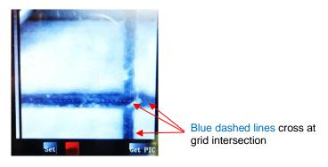
• After clicking on **Home**, press down on the engraver and verify, once more, that the correct grid intersection was used. Back in SCAL, click on **Cut** and the engraving process will be carried out.:
