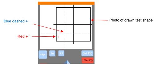
(7) Tap your finger near the middle of the drawn test shape. This will move the red + to that location. Then press **OK**. A new photo will be taken:
