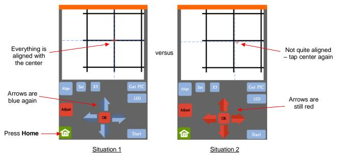
(10) Once the alignment is in place and the arrows have turned blue, press the **Home** button and then press **Stop** on the **Main Screen** to save the calibration and conclude the process:
