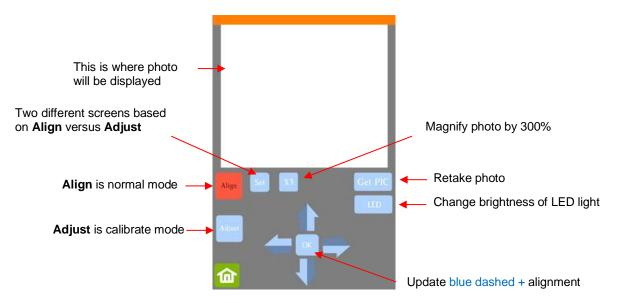
(6) Press **Adjust** to switch to calibrate mode and a new **Start** button will appear in the lower right corner of the **Camera Screen**:
