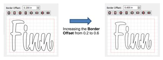
• **Border Options**: These icons can be used to add additional cut lines inside the outer weed border. Each icon in the following screenshot indicates where the lines will be added but a description and example are also shown. Note that once you select an option, you can click at the desired location on the preview image to add the cut line or lines:
