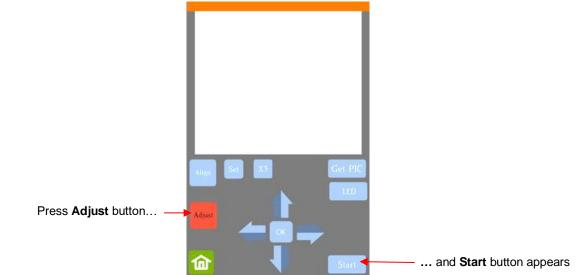
(6) Press Start. A test shape, which is a square with a + inside, will be drawn by the right side pen on the paper and the camera will move over the test shape, take a photo, and display the photo on the control panel. If you cannot see the test shape clearly, press the LED button once so that it reads LED 50% and press the Get PIC button. You should see three items in the photo: the test shape that was drawn with the pen, a red +, and the blue dashed +:
