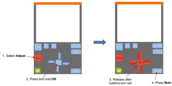
(7) Press Start. The test shape, which is a grid of 6 lines, will be drawn on the paper and the camera will move over the test shape, take a photo, and display the photo on the control panel. If you cannot see the test shape clearly, press the LED button once so that it reads LED 50% and press the Get PIC button. You should see three items in the photo: the test shape that was drawn with the pen, a red +, and the blue dashed +:
