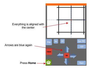
(12) Once the blue arrows appear, press the **Home** button and then press **Stop** on the **Main Screen** to save the calibration and conclude the process:
