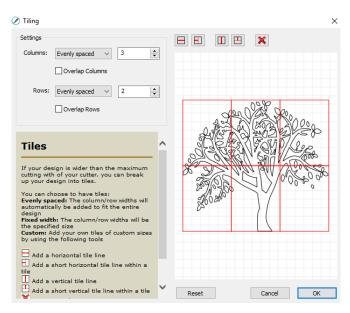
After clicking on OK, but before sending the design to cut, make the Cutting Mat dimensions fit the design. If . any of the design extends beyond the boundaries of grid, those tiles will not cut.
