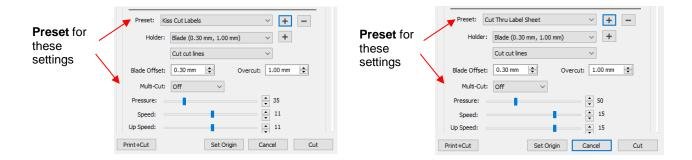
• On the **Style Panel**, select each pair of layers and assign the required **Preset** to that pair:
