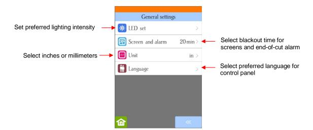
• LED set allows you to change the brightness of the light inside the Skycut or even turn it off:
