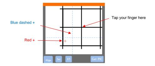
(9) Tap your finger near the middle of the drawn test shape on the screen. This will move the red + close to that location:
