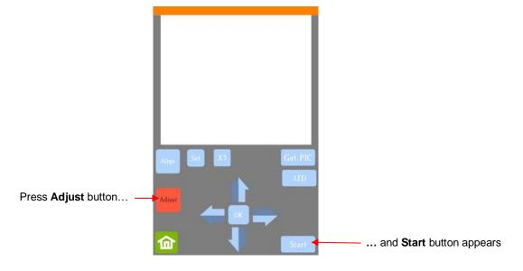
(7) Press Start. The test shape, which is a square with a + inside, will be drawn on the paper and the camera will move over the test shape, take a photo, and display the photo on the control panel. If you cannot see the test shape clearly, press the LED button once so that it reads LED 50% and press the Get PIC button. You should see three items in the photo: the test shape that was drawn with the pen, a red +, and the blue dashed +:
