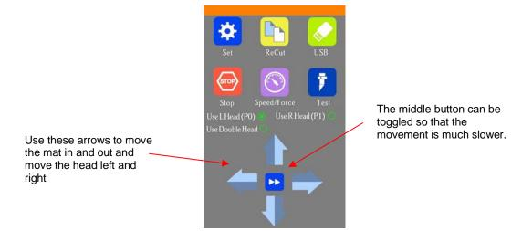
Click on the buttons or the arrow keys on your keyboard to move the head left or right and the mat in and out. The goal is to have the tip of the pen close to the lower right corner of the paper:
