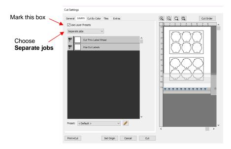
Mark the option for Use Layers Presets and select Separate Jobs. Click on the Print + Cut button and the print and cut process can be carried out as normal. Watch for the job prompt windows to pop up and follow all instructions.
