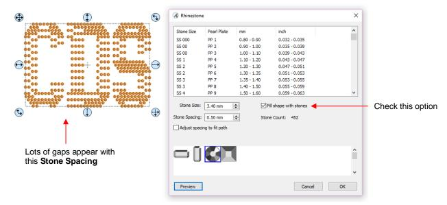
The gaps in the design can be easily corrected by adjusting the Stone Spacing. Instead of 0.50, the spacing is increased slightly to 0.51 mm. The result is a complete correction of the spacing and the design looks great:
