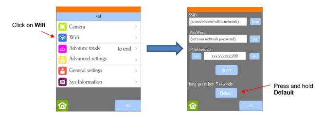
• To reset the Skycut so that it will be found as an available network, press and hold the **Default** button for 3 seconds. Release and you should see the **Apply** button now displays **Wait**. In a minute the **Apply** should return and you can then proceed back to *A* and use the same procedure as if the Skycut was never set up on a network.
