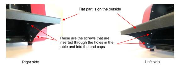
Insert the screws previously removed through the aligned holes and screw back into place. Then repeat on the other side of the cutter.
