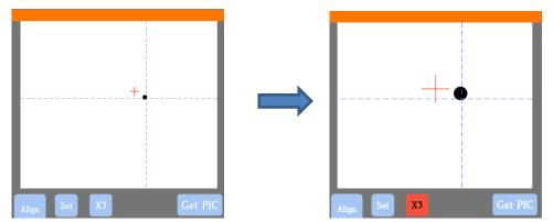
(8) Use the arrow buttons to move the red + as close as possible to the center of the origin target:
