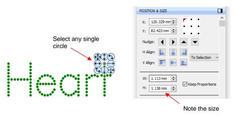
• The circle size in this case is 1.138 mm but let's say the size needs to be 3.4 mm in order for the template holes to work with the SS10 rhinestones purchased. The **Scale** factor is always calculated as:
