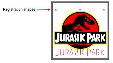
• The layer is selected and the **Cut Line Type** for this layer is changed to **Color Layer Alignment**:
