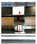
Wheels should be centered over grit shafts which are directly below the white rectangles
