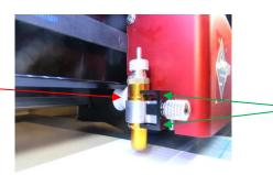
With the front screw loose, the black piece can be moved back just a little bit to allow the blade holder to drop down.
