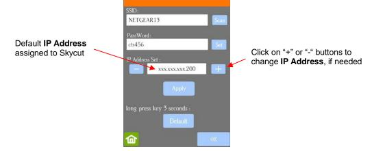
(6) Next check the IP Address that will be assigned to the Skycut. The Skycut will automatically pick up the first three sets of digits from your router but will continue to display them as shown above. You only need to decide if the last set, which should be defaulting to "200", can be used. Use the "+" or "-" buttons to make any needed changes.
