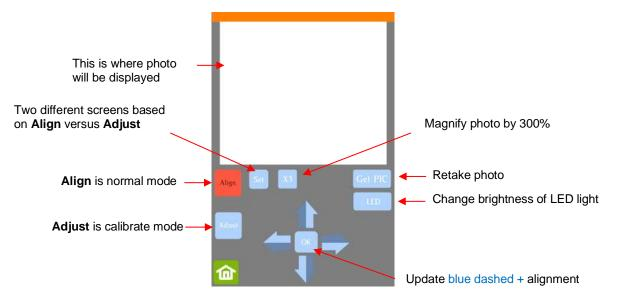
(6) Press **Adjust** to switch to calibrate mode. Press and hold the **OK** button for several seconds until it and the arrows around it turn red (if the buttons do not turn red, please refer to *Appendix D3*):
