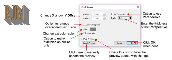
X Offset: Increasing X Offset will extend the extrusion to the right while decreasing it will retract the extrusion towards the left. Note that Y Offset has been set to 0 and Depth is at the default of 0.5:
