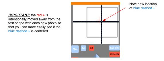
(12) If necessary, repeat Steps 10 and 11 until the blue dashed + is near-perfectly centered in the test shape.
