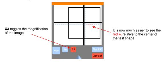
(9) Use the arrows keys to move the center of the red + to the center of the test shape:
