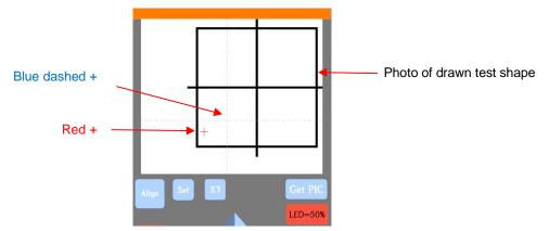
(8) Tap your finger near the middle of the drawn test shape. This will move the red + to that location. Then press **OK**. A new photo will be taken:
