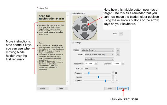
(17) Click on **Scan** and the Skycut's camera will now move over each registration mark and take a photo and make an adjustment. Once it has read all four marks plus the first one a second time, it will proceed to cut out the printed shapes. That's the process!
