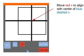
(13) Press OK and the camera will move to the left side test square and will post an image. Repeat Steps (7) –
