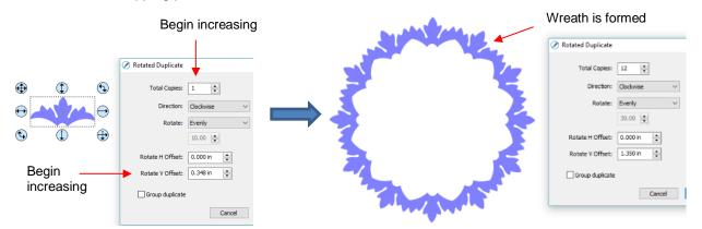
• After creating the pattern, go to Path>Union to remove the overlap and the shape is ready to cut.
