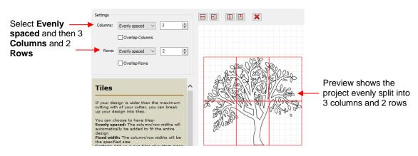
Fixed width: Enter a specific width for the columns. This is probably the most useful choice since you should know the dimensions of the material being used. For example, if you have 12" wide vinyl, then you will probably want the columns to be no wider than ~ 11" or, possibly, 11.5". Also, let's say your vinyl is in 24" long pieces:
