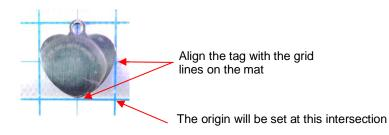
• Load the mat into the Skycut and be very precise in alignment by using the ruler to make sure the mat is perfectly straight:
