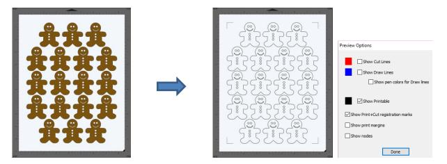
When using Mark inset from print bounds, you may need to turn on Borderless printing in your printer properties window. This can introduce a problem with the reg marks being relocated so you'll also need to locate a setting called Extension or Expansion or Overspray and make it the minimum setting.
