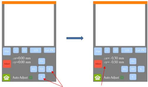
Use these buttons to adjust the  $\Delta x$  and  $\Delta y$  offsets to these
