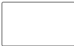
Offset is too low: corners are rounded
