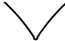
Offset is too high: Divots will appear around corners
