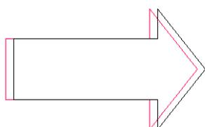
**Red cut line** is 1mm left of the black line: increase X from 21.5 to 22.5
