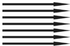
Alternate Line Direction: not marked Tool only travels in one direction
